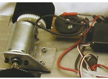
An alternative to the use of resistors, which draw current from the battery, is to develop an electronic speed controller for yourselves.
